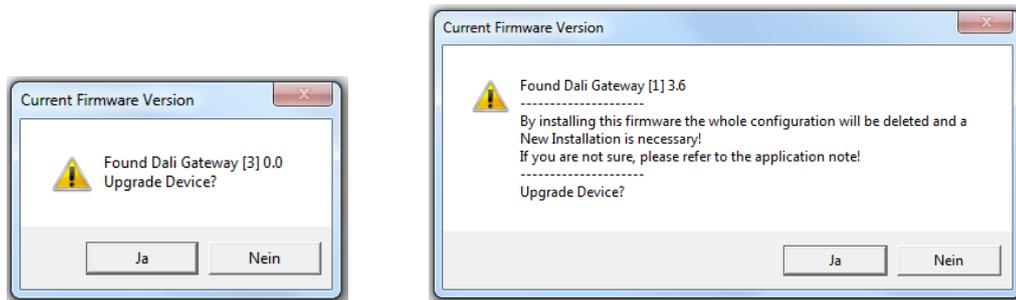
After an acknowledgement, the firmware data will be transferred to the device memory via FTP. A progress indicator informs about the current status of the transfer. Once the update files have been successfully transferred, the device is automatically re-set.
