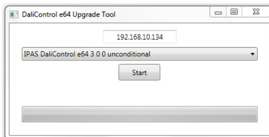
To start the update, enter the IP address of the device that you would like to update. Double-click on the displayed IP address (here 192.168.10.134) to open the entry field.
