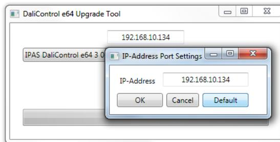
You can now edit the IP address and ensure it is correctly set to the required value. After pressing the OK button, the address is shown in the main window. Before you start the update, please select the required update type from the pull-down menu. The following types are usually available:
