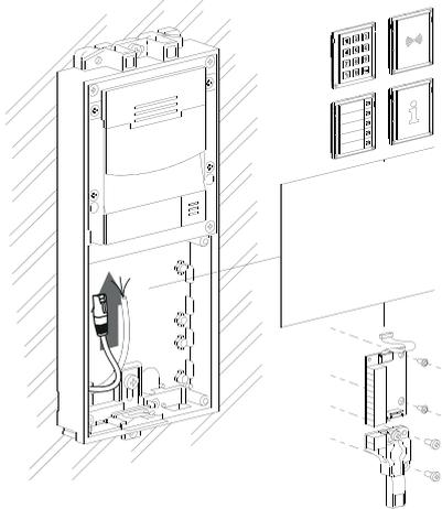
**4** Fix the blind panel (or additional modules that remain in sight) with the supplied screws and put the labels with captions next to the buttons.
