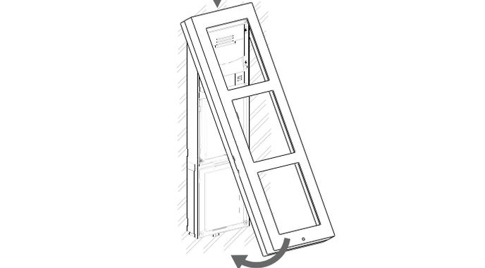
**6** Fix the frame using by the supplied Allen key.
