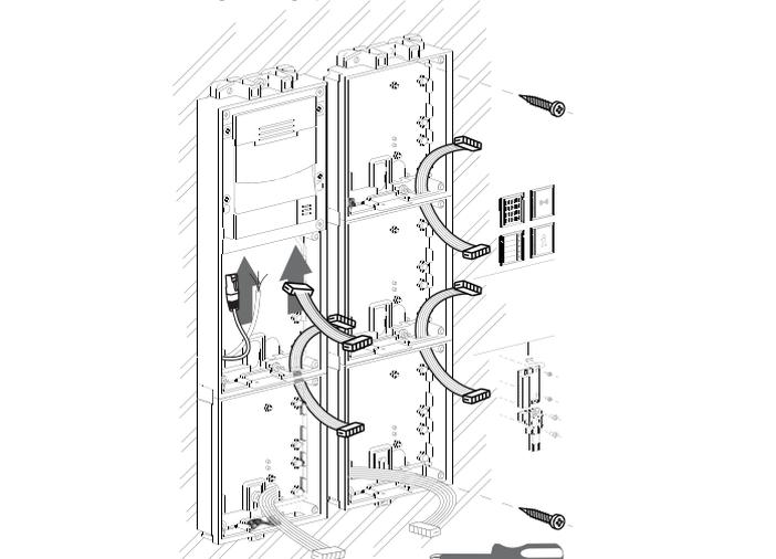
**5** Interconnect the additional modules with the bus as indicated in the schema and then fix the additional modules with the screws.
