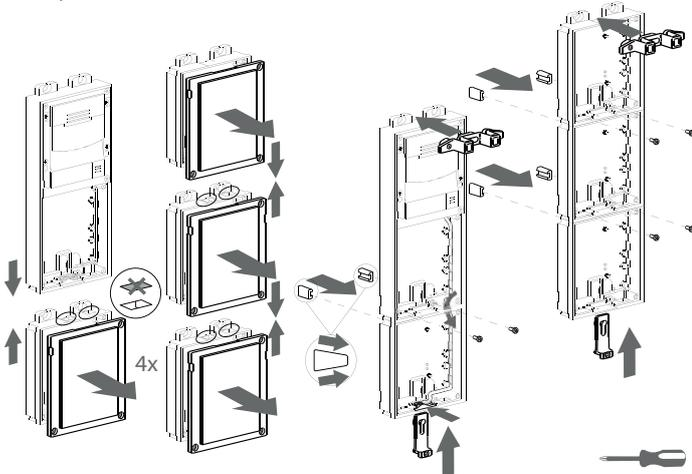
**2** Place the left assembly correctly leveled on the wall and drill two holes for the expansive plugs. Recover the cables, place the bus and fix the left assembly with the screws (included).
