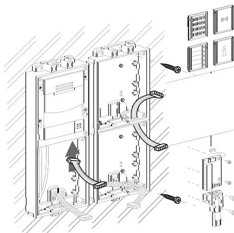
**5** Interconnect the additional modules with the bus as indicated in the schema and then fix the additional modules with screws.
