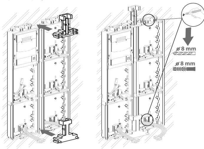
**4** Fix the right assembly to the wall with screws. Make the connections of the basic unit and prepare the additional modules. Pass the bus cable through the gaps.
