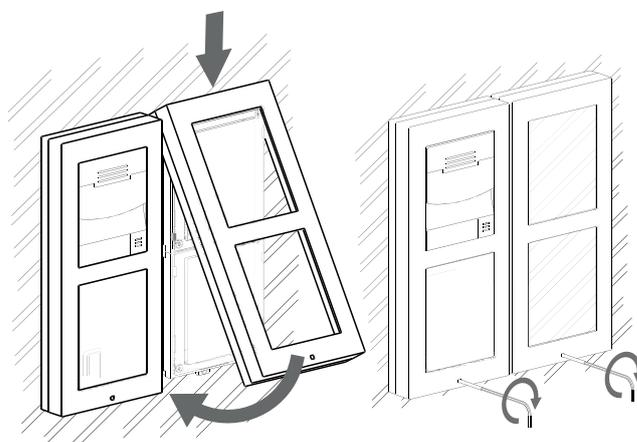
**Note:** it is recommended to install the backplate (ZVP- BP2W2H) if the wall surface irregularity is greater than 0.5mm.
