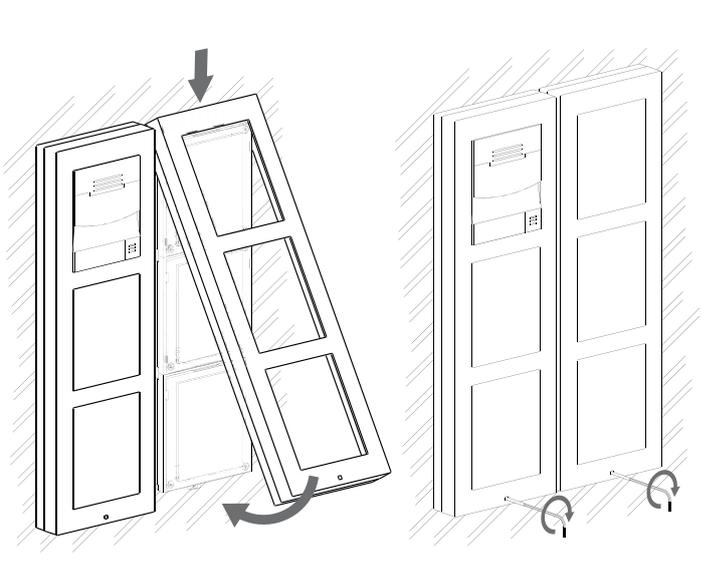
**Note:** it is recommended to install the backplate (ZVP-BP2W3H, ZVP- BP3W3H) if the wall surface irregularity is greater than 0.5mm.
