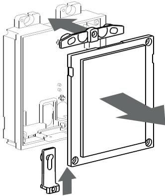
**2** Place the additional module enclosure correctly levelled on the wall and drill two holes for the expanding plugs. Recover the cables and fix the enclosure with the screws (included).
