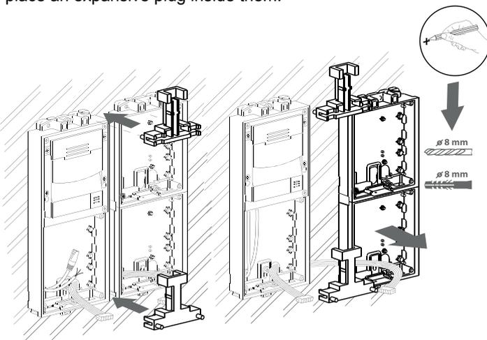
**4** Fix the right assembly to the wall with screws. Make the connections of the basic unit and prepare the additional modules. Pass the bus cable through the gaps.
