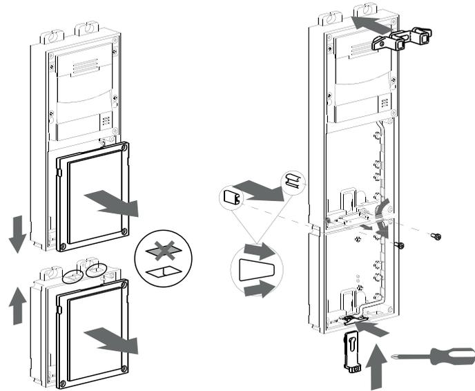
**2** Place the basic unit correctly leveled on the wall and drill two holes for the expanding plugs. Recover the cables and fix the module with the screws (included).
