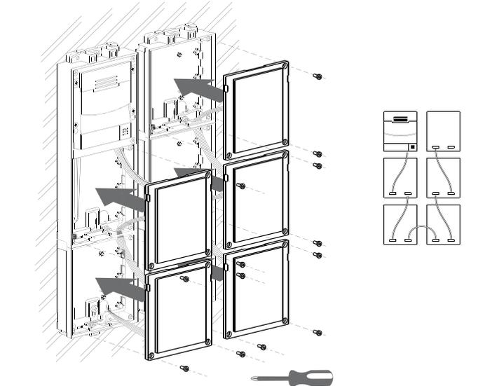
**6** Place the frames and fix them by using the supplied Allen key.
