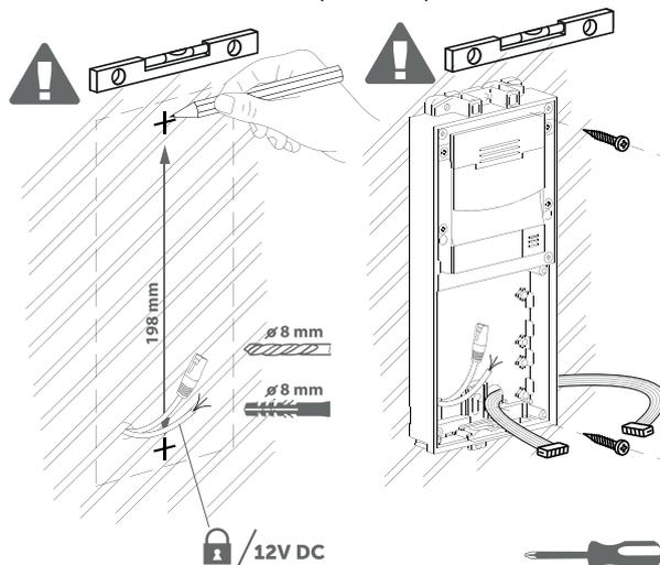
**3** Place the right assembly on the wall by using the T-shape parts. Mark the position of the holes, drill them and afterwards place an expansive plug inside them.
