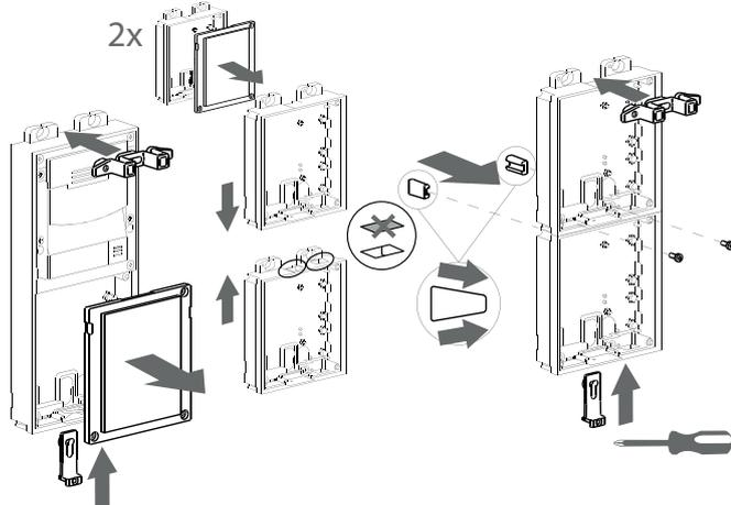
**2** Place the left assembly correctly levelled on the wall and drill two holes for the expansive plugs. Recover the cables and fix the module with the screws (included).
