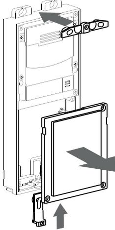
**2** Place the basic unit correctly levelled on the wall and drill two holes for the expanding plugs. Recover the cables and fix the module with the screws (included).
