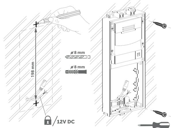
**3** Connect the cables to the basic unit and interconnect the additional modules with the bus.
