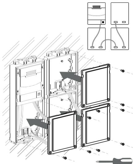
**6** Place the frames and fix them by using the supplied Allen key.
