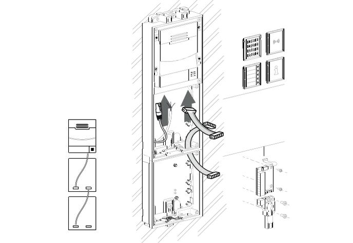
**4** Fix the blind panel and additional modules that remain in sight with supplied screws and put the labels with captions next to the buttons.
