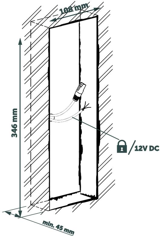
**2** Install the auxiliary parts for the flush-mount assembly.
