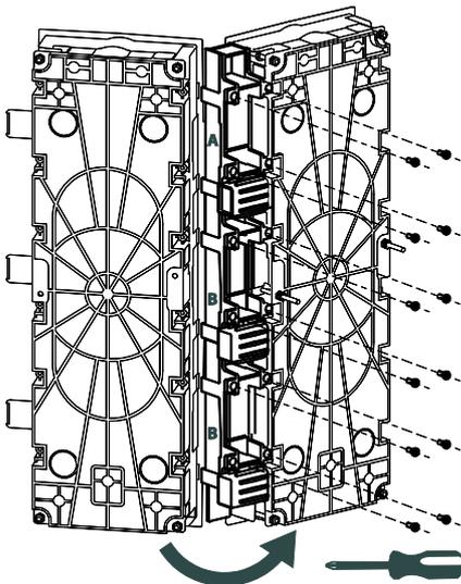
**4** Install the auxiliary parts (A and B) as shown in the figure below.
