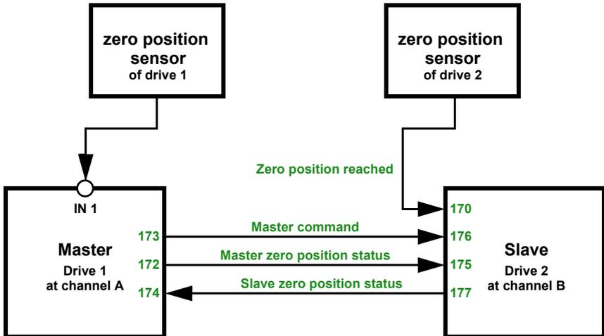
**Actuator A is Master, zero position sensor via bus,
