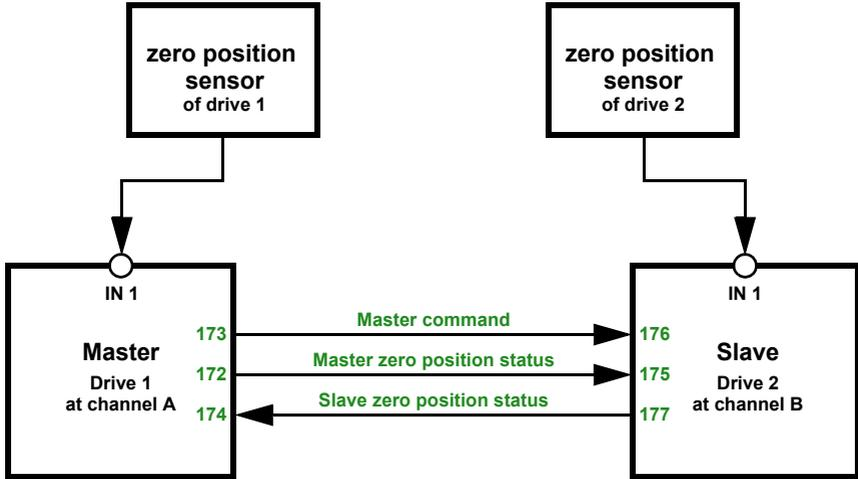
**Actuator A is Master, zero position sensor at input 1 of the actuator,
