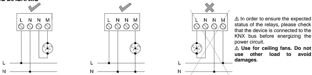
Figure 2: Wiring diagram of a fan
