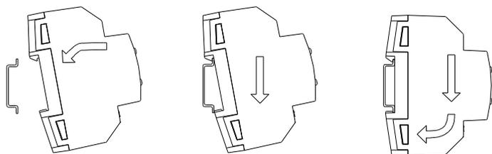
Removing FANinBOX 230V 1CH from DIN rail:
