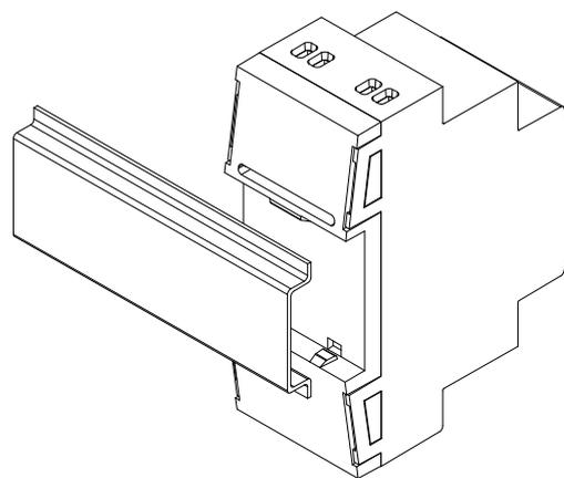
Figure 3: Mounting FANinBOX 230V 1CH on DIN rail
