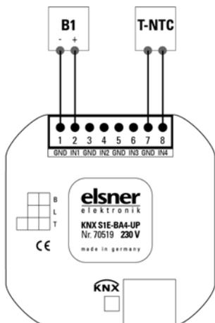
*Example KNX S1E-BA4-UP with binary contact on input 1 and T-NTC temperature sensor on input 4.*
