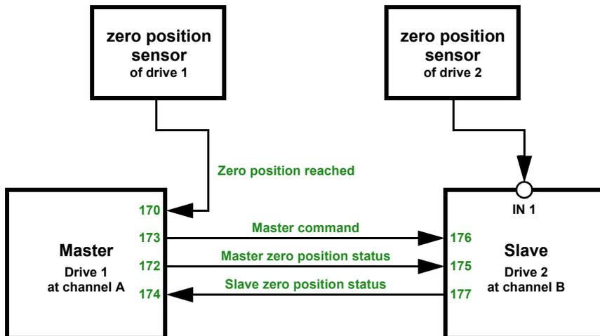
**Drive channel A is Master, zero position sensor via bus,
