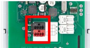
If there is a cavity behind the device, e.g. when using a socket, you can use the red/black KNX bus terminal for connection.
