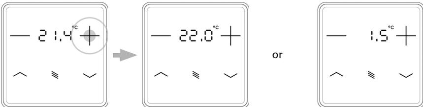
Touch the **+ or -** button briefly: The current **target temperature** (or the basic setpoint shift) is displayed.
