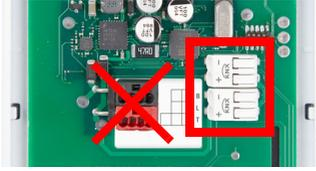
Remove the red-black KNX bus terminal, it is not required.
