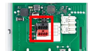
If there is a cavity behind the device, e.g. when using a socket, you can use the red/black KNX bus terminal for connection.
