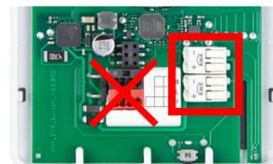
Remove the red-black KNX bus terminal, it is not required.
