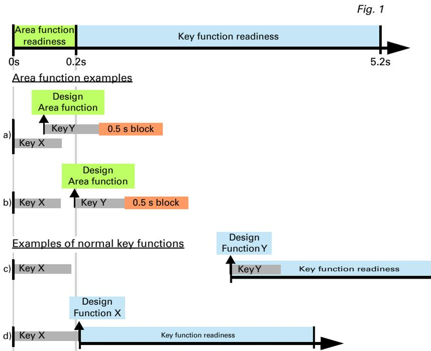
If the area function in the ETS is disabled, the keys can be used normally at any time.
