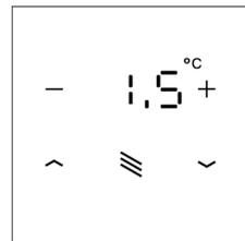
Touch the **+ or -** button briefly: The current **target temperature** (or the basic setpoint shift) is displayed.
