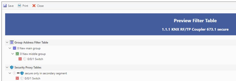
The filter table can be extended by manually adding group addresses. For this purpose, “Pass through Line Coupler” must be activated in the properties window of the corresponding group address.
