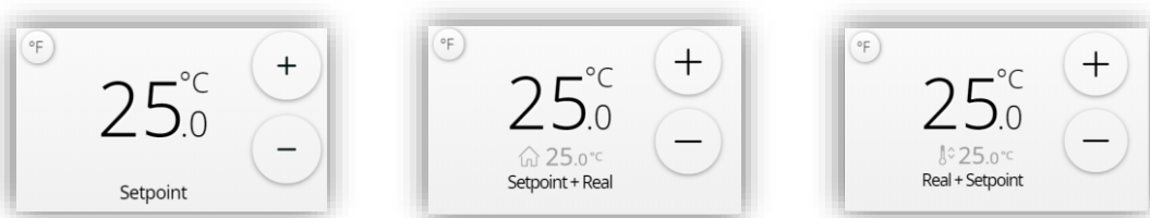
Figure 98. Setpoint Temperature with different indicator types
